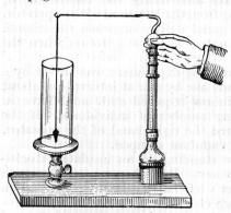
Briefly, it consisted of a vertical mahogany pillar fixed to a platform of solid mahogany; the top of the pillar ended in a brass cap from which projected a horizontal arm of brass. From the end of this arm an ebony ball was suspended by a single thread of unspun silk. Immediately below the pendulum was a disc, also of mahogany, covered by a piece of plate glass about 4½ inches in diameter. For protection
